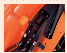
FST Fully Synchronised Main and Shuttle Transmission
