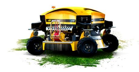
The SPIDER ILD02 is equipped with a four-blade mowing mechanism that ensures perfect mowing and precise mulching making it ideal for golf courses and other sports grounds. For frequent mowing of recreational areas and lawns we offer s-curved cutting blades.
