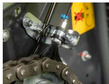
Automatic chain lubrication is standard on BF3500.
