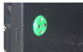
Moisture sensors located inside bale chamber.
