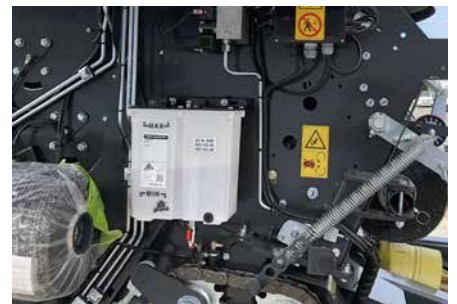
Rigid steel pipes for hydraulic circuits.
