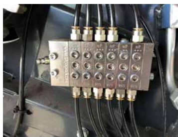
Remote grease bank for bale chamber roller bearings.
