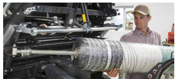
Very low loading height and easy threading of the system make for minimum downtime and maximum time baling.
