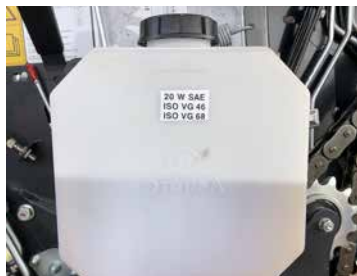
Large capacity chain lube tank.
