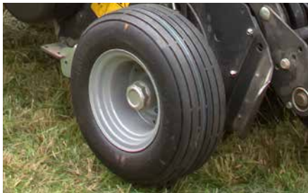
Generous flotation tyres with simple height adjustment.
