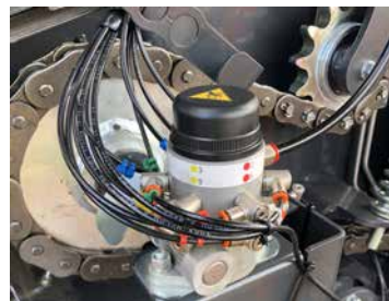
Automatic chain lubrication with individually adjustable outlets.
