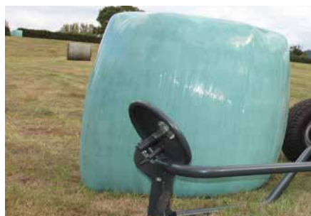
The Kubota WR1850 can be fitted with a bale on end kit.
