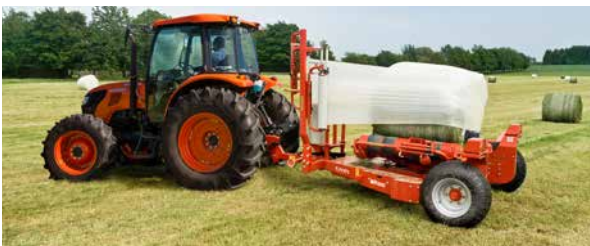
The low mounted table design allows high rotation speed.
